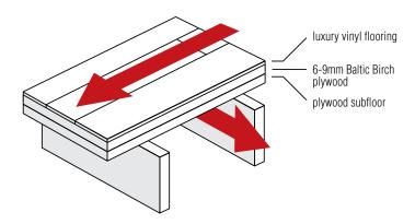
6. For Glue Down Application Sheet wood sub floor with minimum 6mm Baltic Birch Underlayment Plywood. Use 9mm if sub floor needs additional rigidity.
