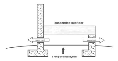
It may be necessary to install temperature/humidity activated exhaust fans to create more air movement in the crawl space. Uncontrolled humidity and moisture in crawl space will lead to mold and damage to the structure, as well as the luxury vinyl floor. In these events, a contractor specializing in dehumidifying systems will need to be contracted to keep crawlspace humidity within proper norms. This is more likely in high humidity areas.
